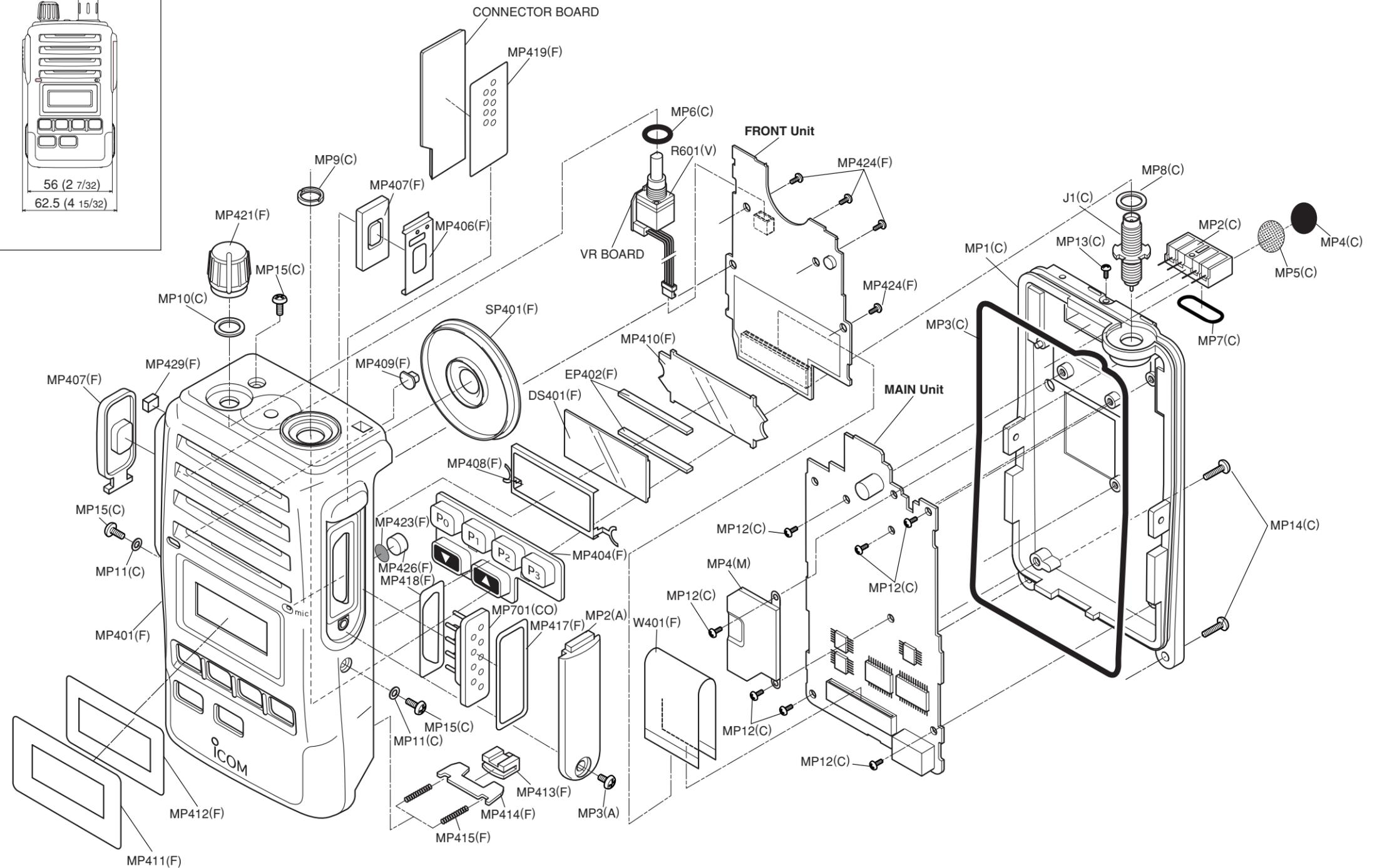
**UNIT abbreviation** (C): CHASSIS PARTS, (M): MAIN UNIT, (CO): CONNECTOR UNIT, (V): VR UNIT, (A): ACCESSORIES, (F): FRONT UNIT
